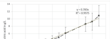
Figure 5: Course of measured (triangle/ grey) and predicted (quadrilateral/ blue) citric acid concentration of batch 7.1 (no part of the training data sets). The average result accuracy of these two runs is 92%.
