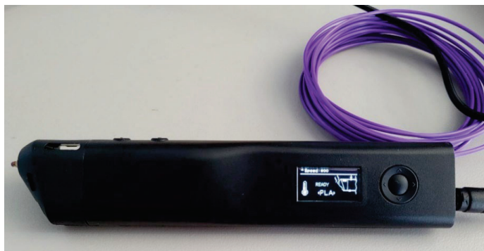
Figure 2. 3D Simo Multipro with settings and purple PLA filament
