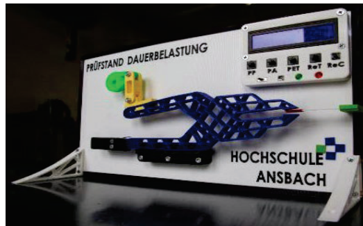
Figure 8. Test device for dynamical testing of the gripper
