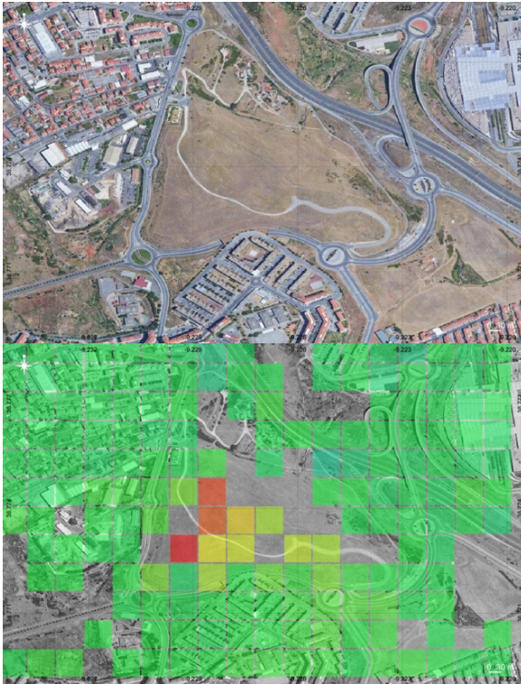
Figure 9. Area of the "Parque das Artes e do desporto" (Lisbon) (top). The area appears to be a large anthropic fill where a slope has been outlined. In the upper area, ground movements away from the satellite of more than 2 cm/year in the LOS direction are observed, possibly related to the consolidation of the fill (bottom).
