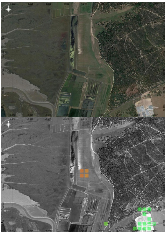
Figure 3. Coastal area on the eastern bank of the Tagus estuary showing a tidal plain occupied by cultivated land (top) A deformation of the terrain in the LOS direction away from the satellite is most likely associated with a subsidence of this terrain (orange pixels: 2-2.5 cm/year) (bottom) linked to the consolidation of the sediment.
