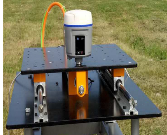
Figure 1. Employed shake table and GPS receiver in experiments.
