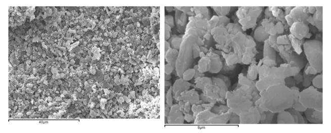
Figure 2. PCM ceramic scaffold after green compaction with black smoke film.
