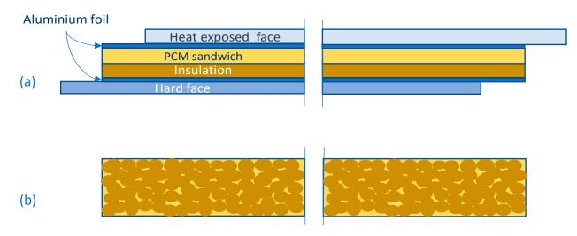
Figure 3. PCM panel design: (a) panel cross section and (b) PCM sandwich.
