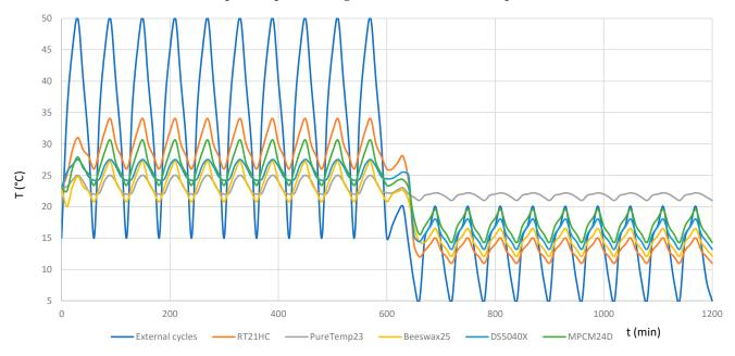
Figure 4. Accelerated Summer/Winter testing cycles.
