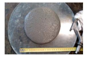
Figure 4. Measurement of the stabilized biscuit.
