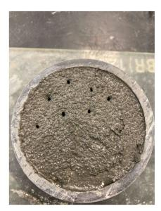
Figure 2. Gap generated in paste indicating the start of setting time.
