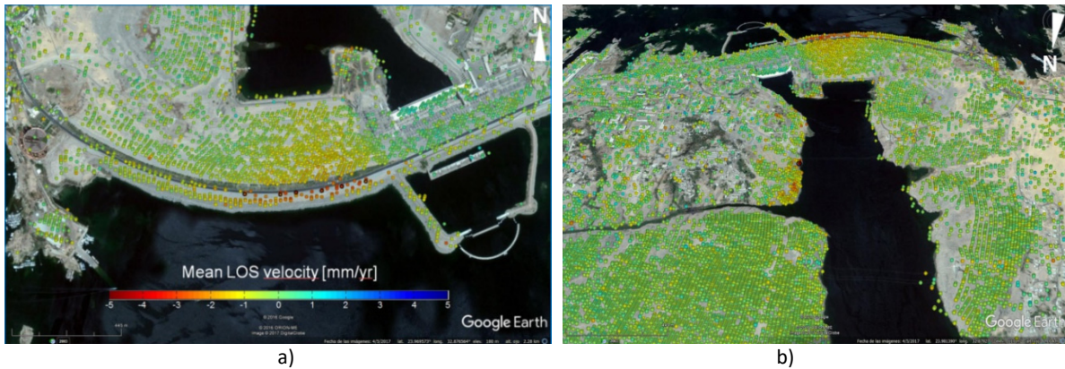
Figure 3. a) Mean LOS velocity derived from Envisat ASAR data over The Aswan High dam (2003-2010); b) Location of a possible landslide 1 km north of the dam (red pixels in the center of the image).
