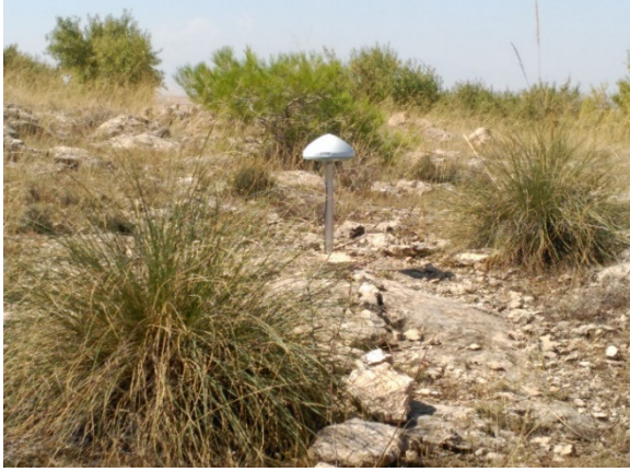
Figure 2. Site 5600 with the GPS antenna AR10 (integrated radome) during a survey.
