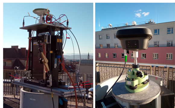
Figure 1. Experiment setup at the rooftop laboratory. Monitoring site with shaker (left), reference site (right).
