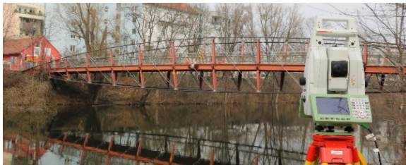
Figure 15. Photo of the measurement setup from the closed by bank, where the RTS was located.
