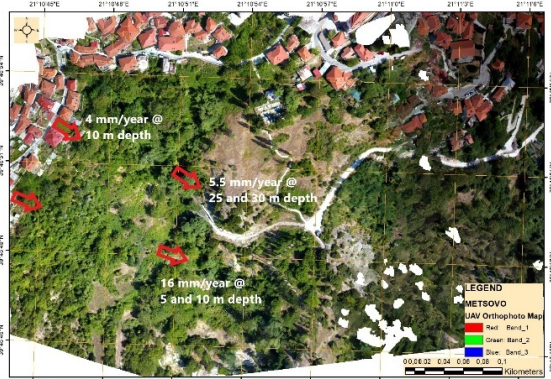
Figure 4. Orthophoto map of Metsovo (the red arrows represent the direction and rate of subsurface movement in mm/year at several depths below the ground surface).
