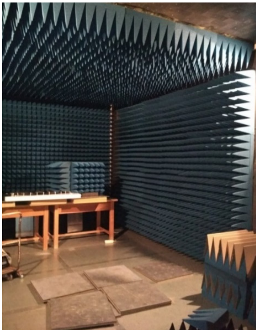
Figure 1. The anechoic chamber of the Laboratory of Wireless and Long Distance Communications, of the School of Electrical and Computer Engineering, NTUA.
