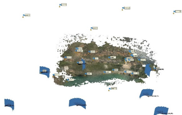
Figure 9. Position of markers and cameras in orientation.
