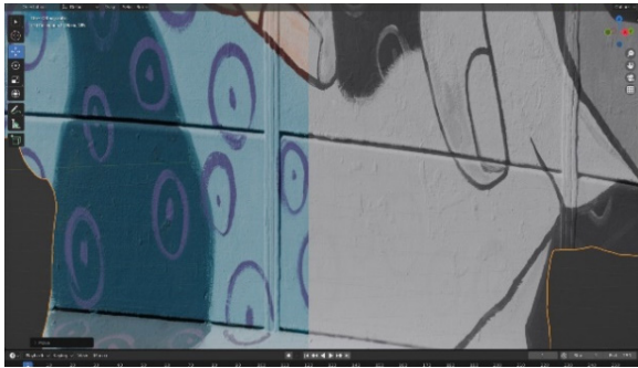
Figure 4. Detail of the multi textured 3D Modell in Blender. Left: VIS texture, right IRR texture. The pigment used for the purple circles has the same characteristics as the blue background under IR.
