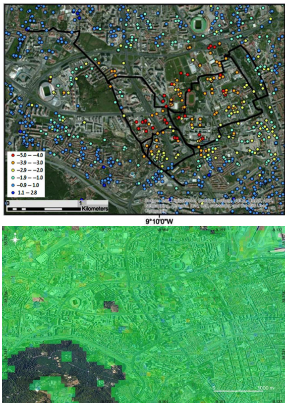
Figure 10. Area of the University of Lisbon Campus with InSAR data obtained from ERS images (from Catalão et al. , 2015) (top). Data obtained from GEP after processing Sentinel-1 images (bottom). The green colour of the pixels indicates stability of the whole area.
