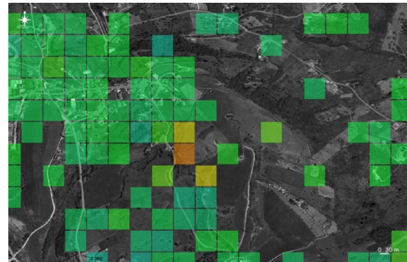
Figure 5. Monte Mourão area (358 m). Ground movement velocities in LOS direction of more than 1.5-2 cm/year (yellow and orange pixels) are observed linked to a known active landslide.
