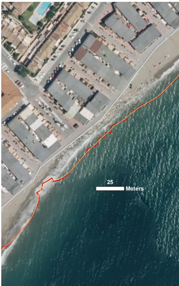
Figure 3. Satellite-derived shoreline from Sentinel-2 (red colour, 2075.39 m length) and the shoreline resulting from applying the smoothing process (yellow, 2019.09 m).
