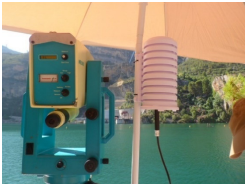
Figure 5. Kern ME5000 Mekometer on pillar equipped with a parasol and a data-logger for dry and wet temperatures as well as air pressure.
