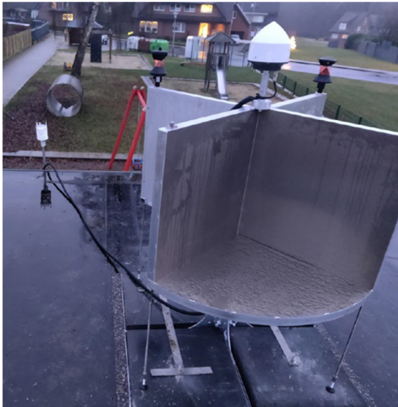
Figure 6. DCR600, Ø1,2m with GNSS-Antenna and weather-sensors. Image courtesy ALLSAT & RAG.
