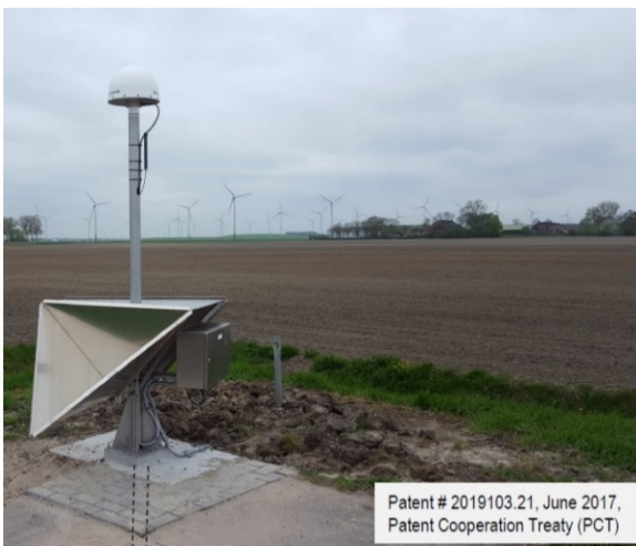
Figure 8. The Netherlands: Integrated Geodetic Reference Station (IGRS). Patented D-CR and GNSS-platform (Hanssen et al. , 2018, page 3).
