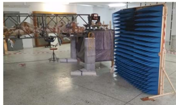
Figure 3. Special barrier surface for the absorption of reflected electromagnetic signals.
