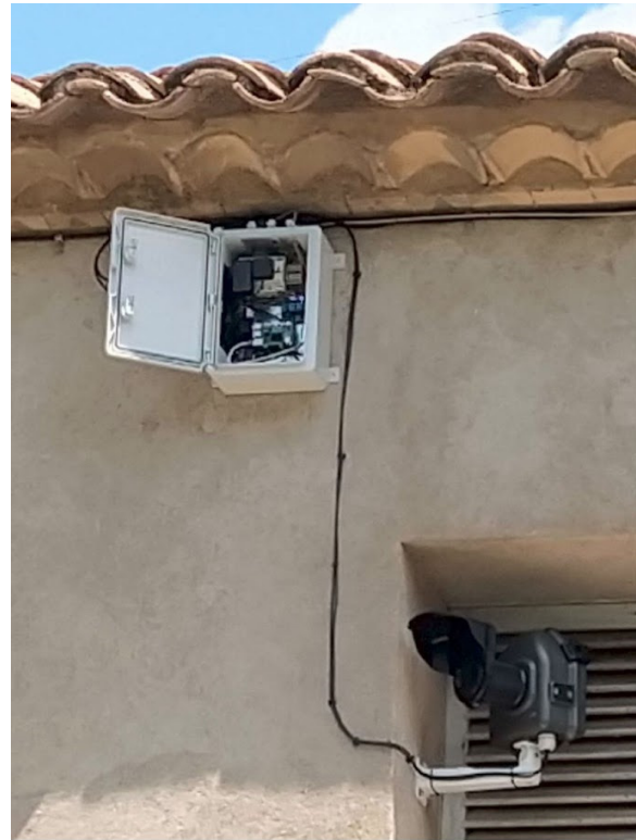
Figure 2. Single camera housing: 1) DSLR camera; 2) USB extender through ethernet receiver; 3) DSLR camera power supply; 4) USB extender power supply.
