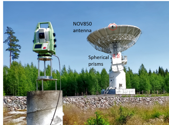
Figure 2. Simultaneous tachymeter and GPS local tie monitoring.
