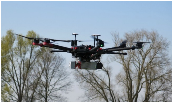
Figure 3. UAV system with the RIEGL miniVUX-SYS.
