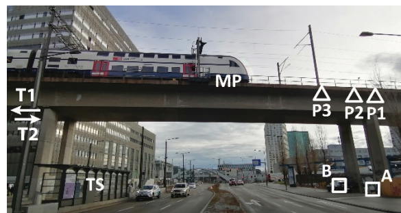
Figure 8. Situation during the bridge monitoring experiment where A and B indicate the two TIDEP-01012 devices, P1-P3 selected areas on the upper soffit, MP and TS a metallic platform and a tram shelter, respectively.
