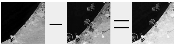
Figure 3. Image Algebra Change Detection: Substraction of pixel-values of two images to identify the differences (FIS, Uni Bonn).
