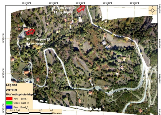
Figure 6. Orthophoto map of Zotiko (the red arrows represent the direction and rate of subsurface ground movement in mm/year at several depths below the ground surface).
