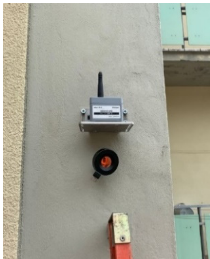
Figure 19. Prism 102B positioned under the TILT-B sensor.
