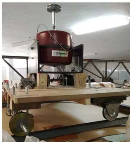
Figure 4. The electric vehicle with the excitation unit placed on it. Its movement was forced along the iron rails shown.
