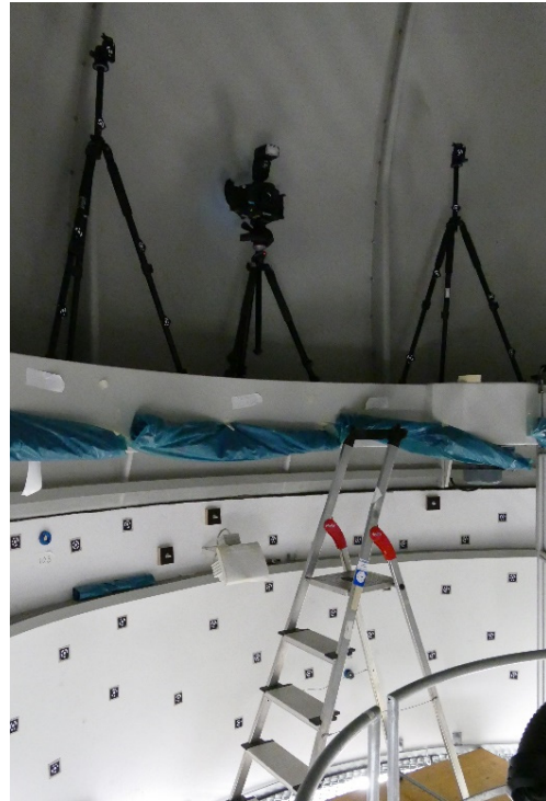
Figure 5. Fixed camera position on a stable tripod for one of eight azimuthal reference positions. Photogrammetric reference points beyond the camera's field of view, for instance under the tripod, are not covered. Image acquisition is performed by remote control.
