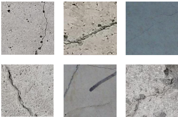
Figure 4. Examples of cracked surfaces ("Positive") - authors' own dataset.
