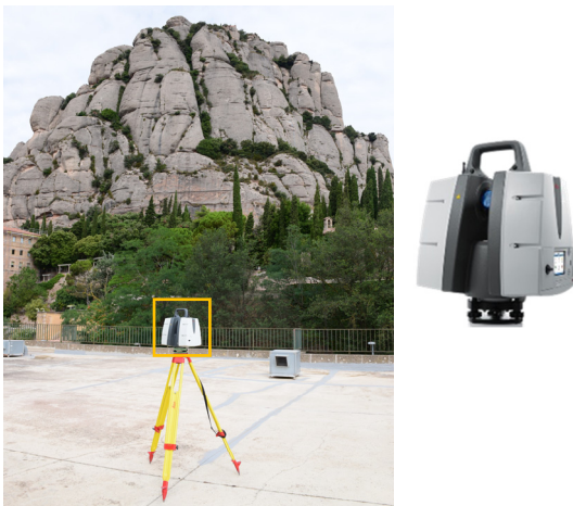
Figure 2. TLS used in the study, Leica ScanStation P50. In the background, the characteristic Montserrat landscape can be appreciated: stepped slopes where vertical conglomerate intercalation of and fine layers of sandstone and siltstone.
