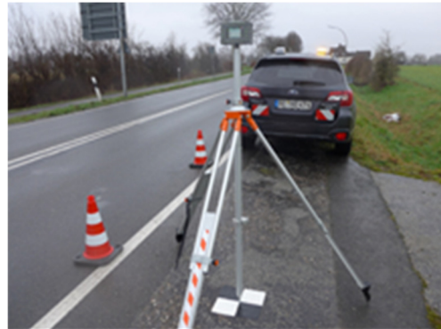
Figure 3. Measurement of ground control points. Image courtesy, RAG.
