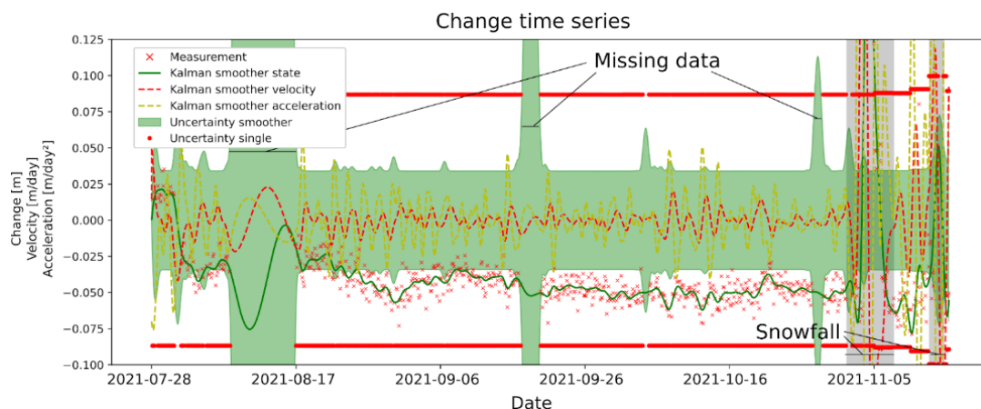
Figure 4. Exemplary time series at a location with subtle, but continuous erosion. Note how data gaps are interpolated, but if they are too long, a ringing effect occurs (as seen in the days before 17-08-2021). A daily pattern can be observed, especially in the velocity and acceleration estimations. Snowfall at the end of the observation period causes large displacement values.
