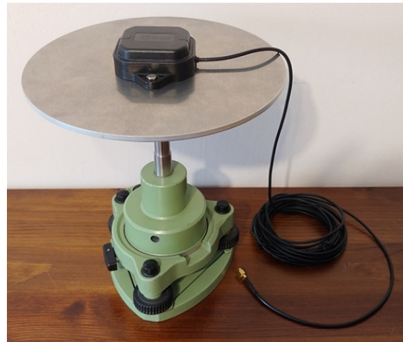
Figure 1. The u-blox ANN-MB-00 antenna with self-made aluminum ground plane.
