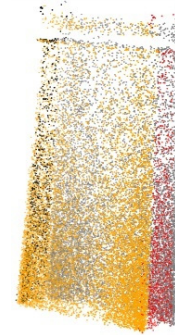
Figure 8. Extractions of planes by using RANSAC-based algorithm for pier 2, four planes are represented by red, grey, orange and black points.
