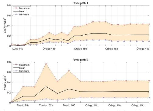
**Figure 5.** Variation of the yearly WEI<sup>+</sup> along the two river paths indicated in Figure 1. The maximum, mean and minimum values are marked in red, black and blue, respectively.
