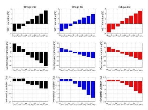
**Figure 11.** Variation of the WEI<sup>+</sup>, available water (WEI<sup>+</sup> denominator) and consumed water (WEI<sup>+</sup> numerator) induced by environmental flow scenarios in three river stretches in the upper (Órbigo 43a), middle (Órbigo 46) and lower (Órbigo 49d) parts of the basin (Figure 3).
