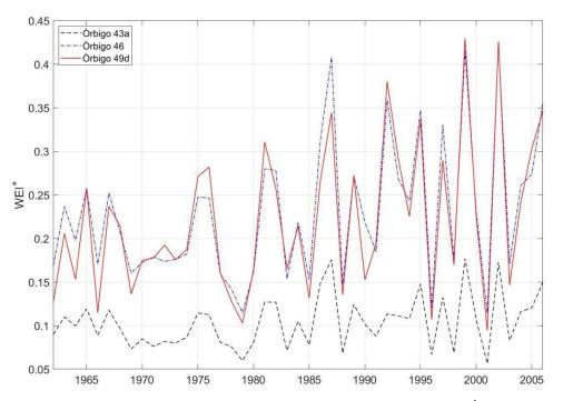
**Figure 6.** Evolution of the yearly WEI<sup>+</sup> in three river stretches in the upper (Órbigo 43a), middle (Órbigo 46) and lower (Órbigo 49d) parts of the basin (Figure 3).
