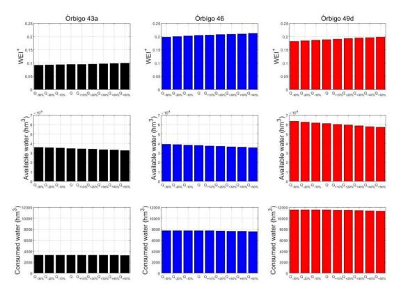
**Figure 10.** WEI<sup>+</sup>, available water (WEI<sup>+</sup> denominator) and consumed water (WEI<sup>+</sup> numerator) for each environmental flow scenario in three river stretches in the upper (Órbigo 43a), middle (Órbigo 46) and lower (Órbigo 49d) parts of the basin (Figure 3).
