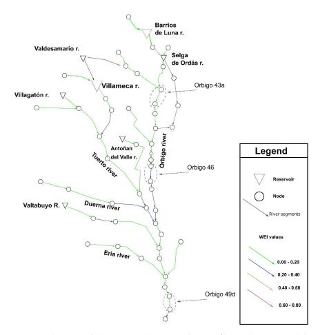
**Figure 4.** Plan view of the water exploitation index (WEI<sup>+</sup>) in each river stretch based on the entire simulated period.
