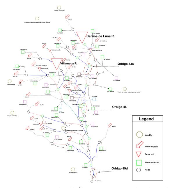
**Figure 3.** Topology of the Órbigo water resources system used in the basin simulation model (SIMGES). The green, pink and blue squares represent agricultural, urban and industrial demand units, respectively. Three river stretches (represented as arrows in the figure) analyzed in this work (Órbigo 43a, Órbigo 46 and Órbigo 49d) are marked in the figure.
