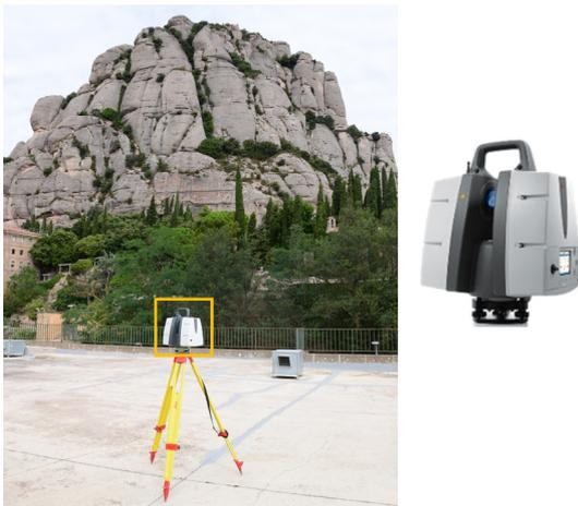
Figure 2. TLS used in the study, Leica ScanStation P50. In the background, the characteristic Montserrat landscape can be appreciated: stepped slopes where vertical conglomerate intercalation of and fine layers of sandstone and siltstone.
