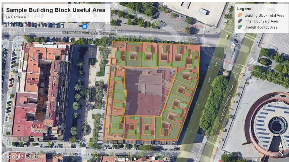
Figure 3.6 Sample building rooftop analysis for PV installation [27].
