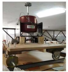
Figure 4. The electric vehicle with the excitation unit placed on it. Its movement was forced along the iron rails shown.
