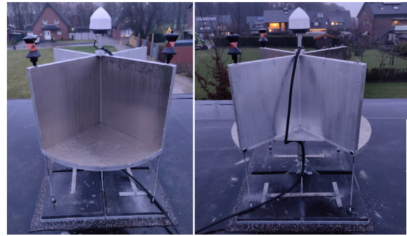
Figure 6. DCR600, Ø1,2 m with GNSS-Antenna and targets. View from west (left) and south (right). Image courtesy ALLSAT & RAG.
