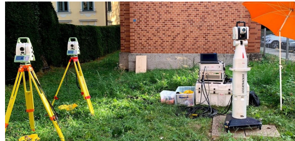
Figure 9. Instrument setup and left wall of aqueduct.
