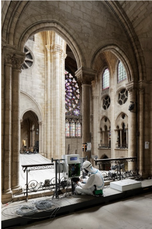
Figure 2. Set-up of the monitoring system of Notre-Dame Cathedral in Paris. ©OSMOS Group SA.
