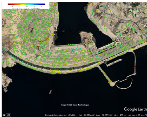
Figure 4. Mean LOS velocity derived from Sentinel-1A/B ascending data over The Aswan High dam (2015-2021).
