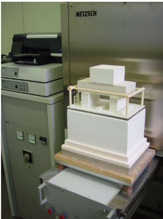
Figure 47. Images of the thermal conductivity NETZSCH TCT 426 at PRTC analytical laboratory. (Top picture) General overview of the accessories; (Left and right bottom pictures) View of the thermal conductivity measurement system by hot wire standard cross method.
