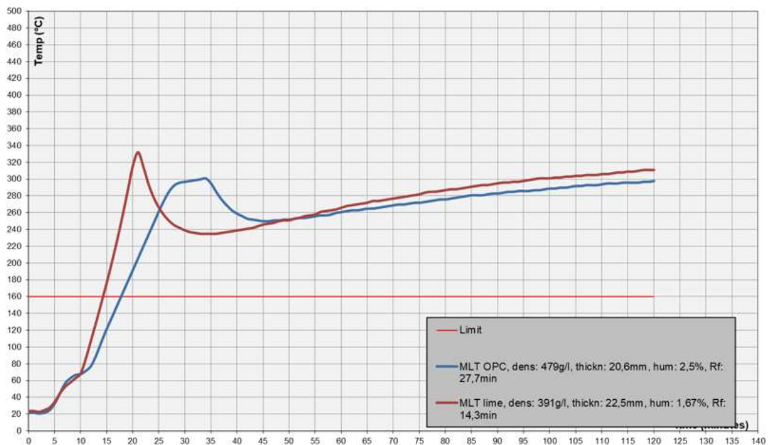
Figure 189. ISO Fire Rate curves of MLT samples using lime and OPC as CaO-source respectively.
