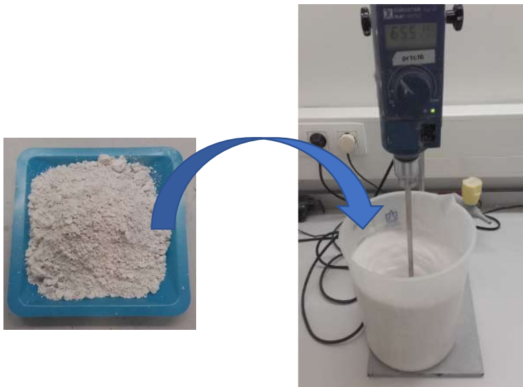
Figure 28. Slaking of lime in demineralized water by stirring in a non-continuous way.
