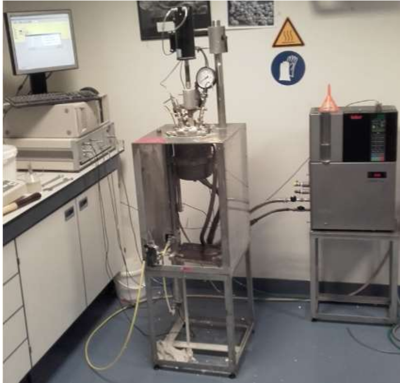
Figure 36. Vertical stirring autoclave reactor system at PRTC laboratory.
