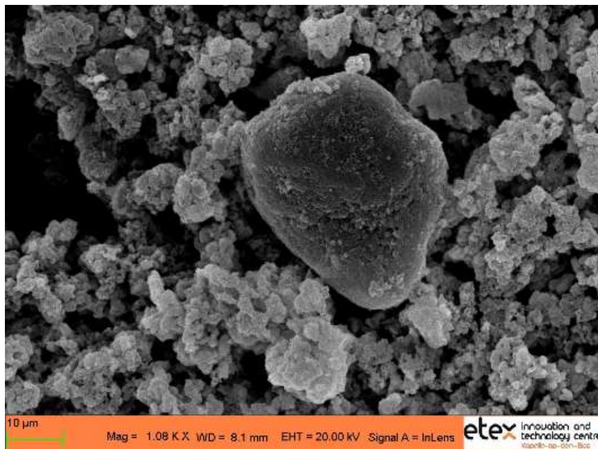
Figure 90. SEM image of GT580, as C-S-H gel preparation stirred at 200 rpm.
