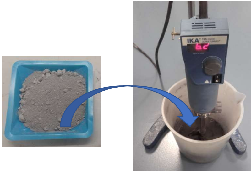
Figure 27. Dispersion of silica fume in water by high shear mixing tool.
