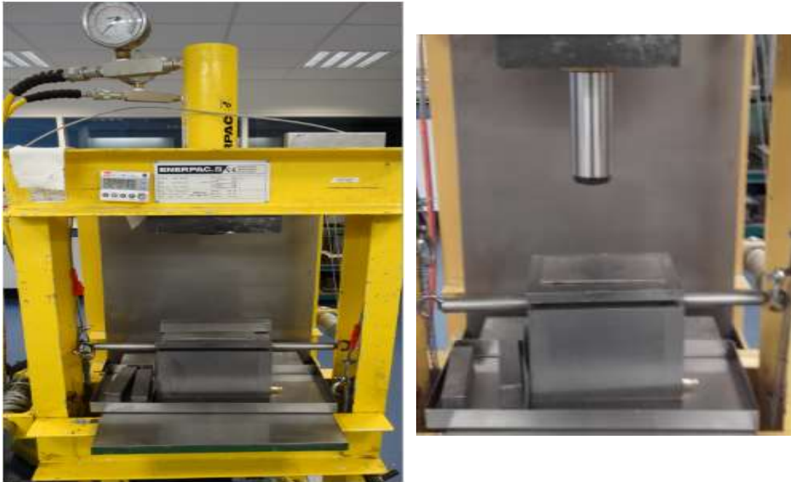
Figure 30. (Left) ENERPAC Hydraulic yellow press, (right) metallic mold with inner filtration holes.
