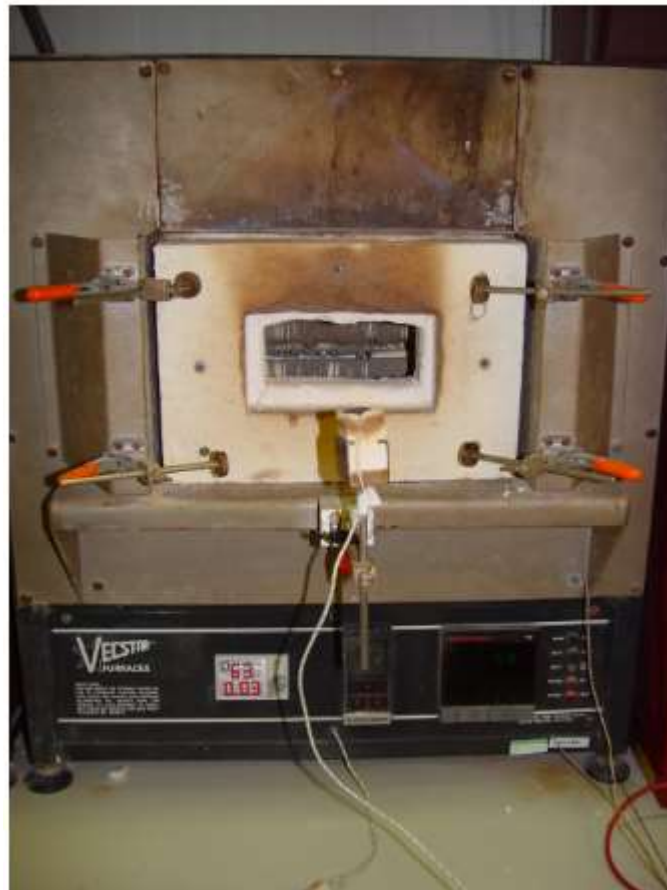
Figure 48. VECSTAR Furnace coupled with a wool glass-frame for the RF Test.
