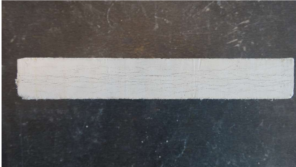
Figure 188. Aspect of MLT-boards made with lime instead of OPC.
