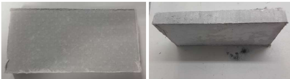
Figure 31. Calcium silicate board after filter pressing. (Left) Top view and (right) side-view.
