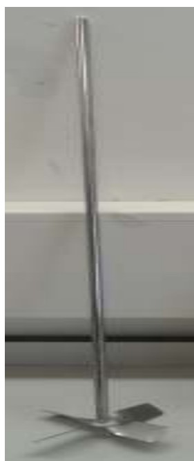
Figure 85. Metal stirrer composed of four curved cross-shape blades used as mixing tool during pre-reaction stage.
