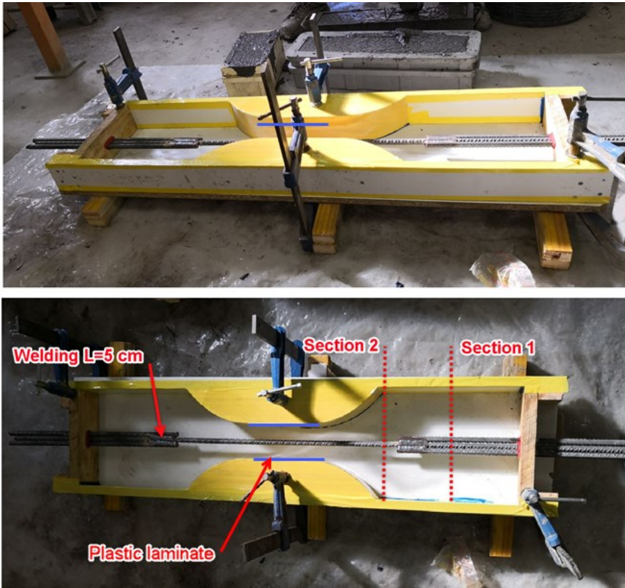
Figure2: Dog bone-shaped specimen and reinforcement detail.
