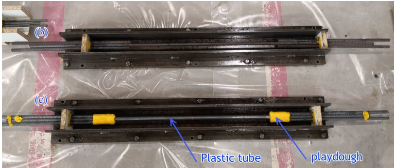
Figure 6- 25: Specimens details for test program 1, (a) general geometry of specimens(b) specimen without plastic tube [bonded], (c) specimen with plastic tube [unbonded].
