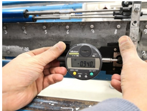
Figure 2-10: DEMEC measurement machine and grid steel discs.
