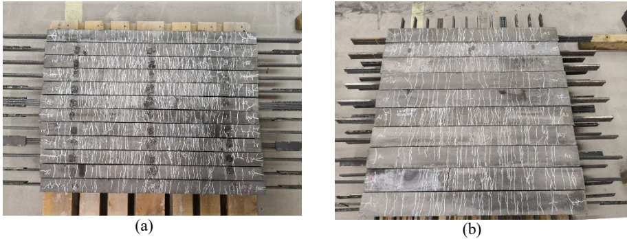
Figure 6- 12: Crack pattern of specimens (a) UHPFRC type C1 (b) UHPFRC type C2
