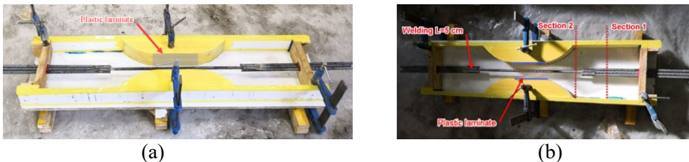
Figure 6- 32: Reinforcement and mold details of dog bone-shaped specimens.
