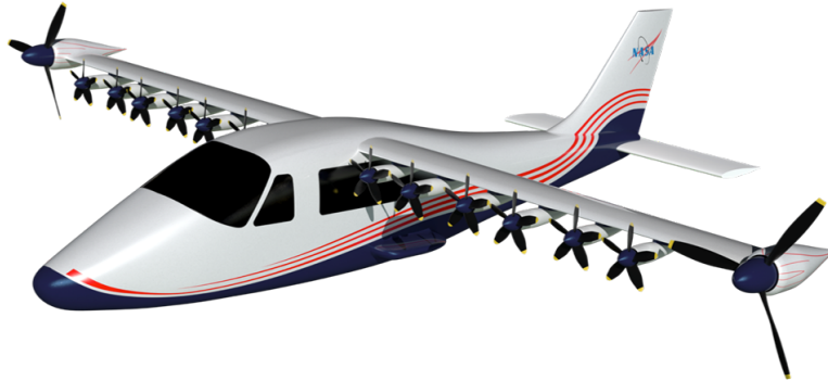
Figure 2.7: Leading edge distributed electric propulsion applied to NASA's X-57 Maxwell aircraft.
