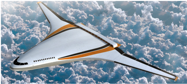
Figure 2.6: Trailing edge distributed electric propulsion with boundary layer ingestion applied to NASA's N3-X aircraft.
