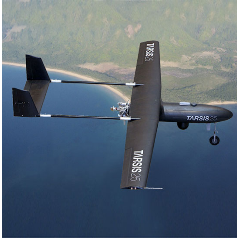
Figure 3.2: RPAS TARSIS 25 manufactured by AERTEC Solutions.
