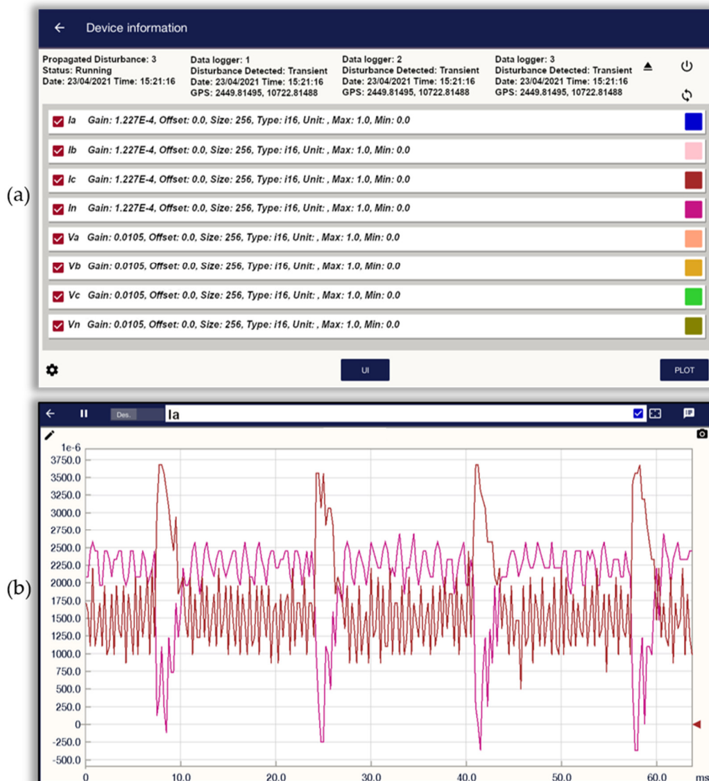
Figure 6. Image interface of the application developed for mobiles to control the proprietary data logger. (a) Measurement control screen and configuration of measurement channels: Ia, Ib, Ic, In, Va, Vb, Vc, Vn. (b) Real-time signal display screen.
