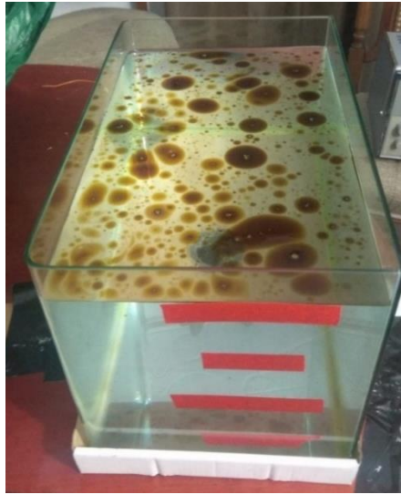
Figure 5.4. Experimental tank with 0.03 \text{ mL}_{\text{oil}}/\text{cm}^2 from gasoline engine at 20 cm height.
