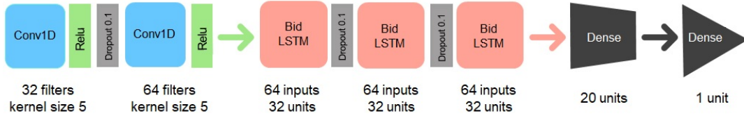
Fig. 6.4: ConvLSTM model architecture used for anomalous diffusion analysis in [10, 17].
