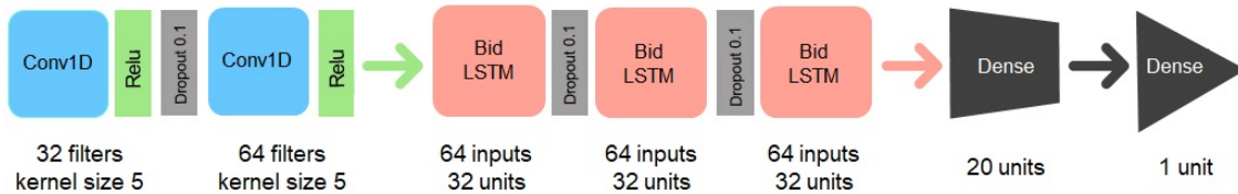
Fig. 7.3: Machine learning used for inferring the generating \mu and \nu parameters of Wu-Baleanu trajectories.
