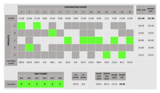
**Figure 6.** Designed HMI interface. Columns represent the evaporation plants. The first row indicates the evaporation load in t/h. The next five rows correspond to the products and the last one displays the cooling water to each SC. Current load assignation arises in the green boxes. Dark gray boxes indicate forbidden connections.
