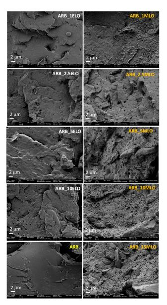
Figure 7. FESEM micrographs of fractured surfaces of ELO- and MLO-modified Arboform formulations.
