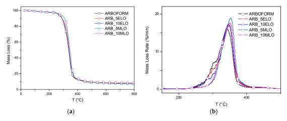
Figure 6. TG (a), DTG (b), DSC curves of ELO- and MLO-modified Arboform formulations.
