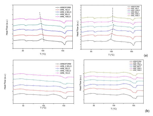
**Figure 5.** DSC curves (1st heating run (**a**) and 2nd heating run (**b**)) of ELO (left) and MLO (right) added formulations.
