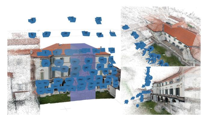
Figure 8 | Close-range photogrammetry of the facade on the Palace garden performed with DJI Mavic mini. Left: the evolution of processes from point cloud to textured model. Right: images of the sparse point cloud highlighting the location of acquired photographs and targets used for model alignment. The UAV acquisition was conducted with the support of licensed pilot R. De Marco.
