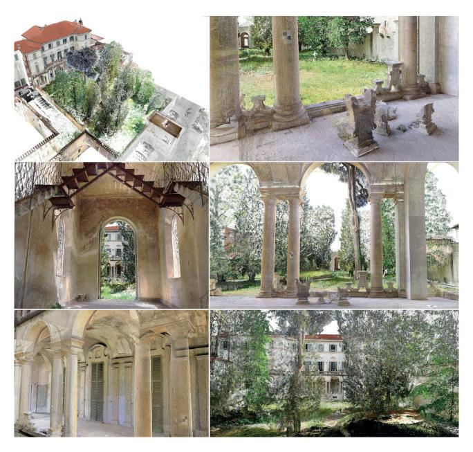
Figure 7 | Images of the TLS point cloud integrated with the point cloud generated by close-range aerial photogrammetry. The point cloud was created by paying attention to fully document the architecture but at the same time to detect the tree species. Numerous scans were taken from high points on the façade and Belvedere to obtain data on the summit portions of the garden as well.
