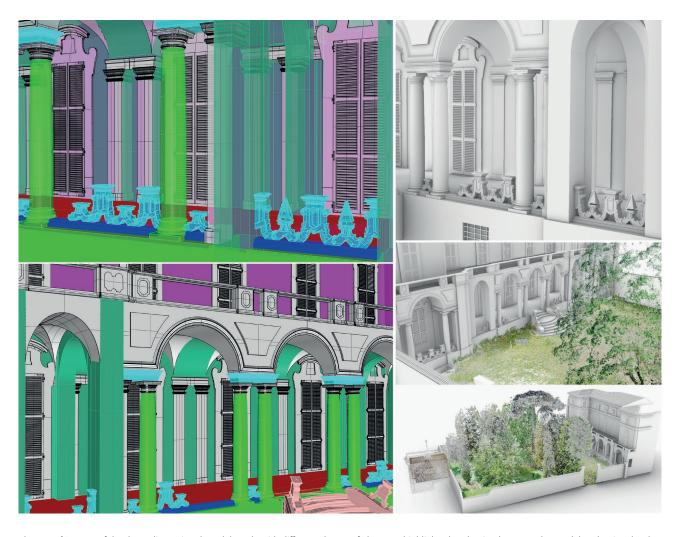
Figure 12 | Images of the three-dimensional model made with different classes of elements highlighted and union between the model and point cloud to verify the reliability and integrate different data. Two-dimensional drawings and models are partly supplemented by the work produced by students of the didactic seminar.
