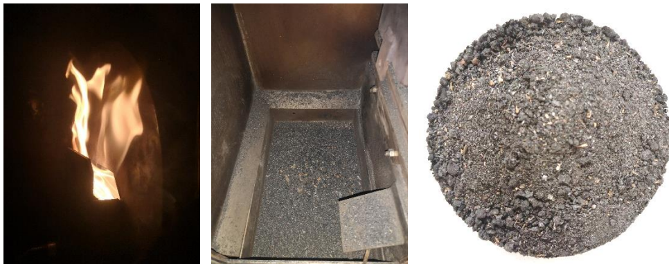
Figure 10. Flame during combustion of pellets of dry BSGs (left), residue into the incineration unit after combustion (middle), and collected ash (right).
