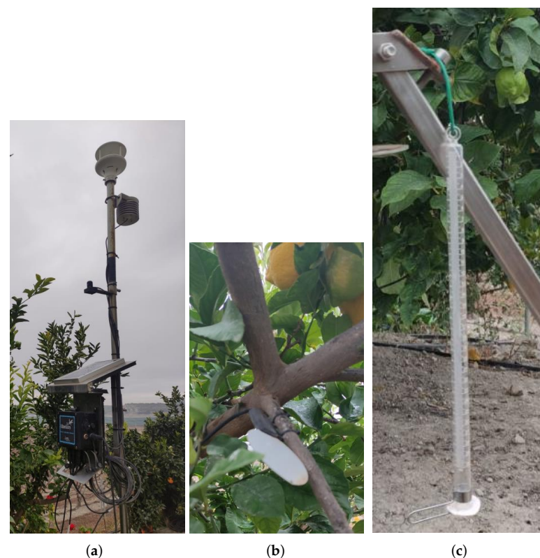
Figure 1. IoT infrastructure deployed for data collection. (a) Overview of IoT sensors deployed. (b) Detail of the leaf vaporisation sensor. (c) Piche evaporimeter model deployed.
