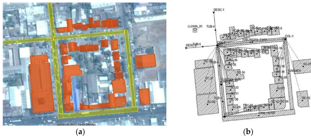
Figure 3. (a) Surface of green roofs (orange areas) and collectors (yellow areas) in Case Study 1; and (b) Hydrological model in SWMM.
