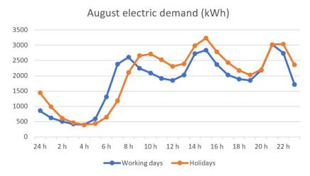
**Figure 3.** Hourly electricity demand for the month of August. Note: vertical axis shows average energy demand in MWh, while horizontal axis the hours of a day.
