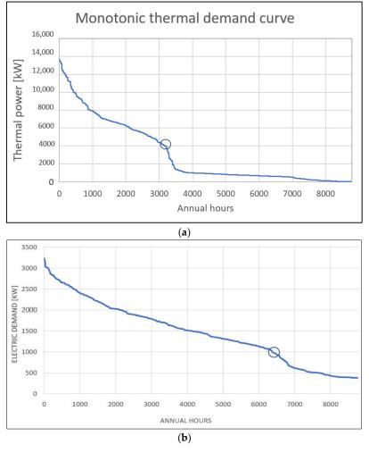
**Figure 4.** Monotonic annual demand curve. Graphical representation of demand during the year. (a) Annual monotonic thermal demand curve. (b) Annual monotonic electricity demand curve.
