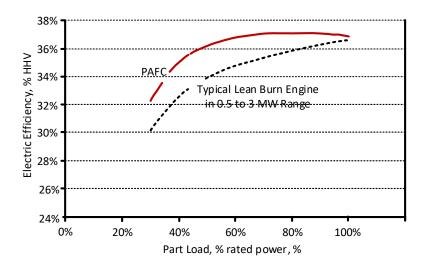
Figure 5. PAFC performance at partial loads.
