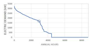
**Figure 7.** Monotonic electricity demand curve: graphical representation of demand in months with cooling demand.
