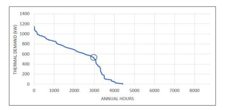
**Figure 6.** Monotonic thermal demand curve: graphical representation of demand in months with heating demand.
