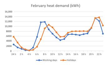
**Figure 2.** Hourly thermal demand for heating and DHW for the month of February. Note: vertical axis shows average energy demand in MWh, while horizontal axis the hours of a day.
