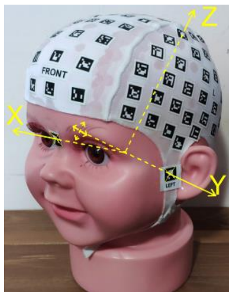
Figure 1. Dummy with the coded cap on. The local reference system (XYZ axes) is displayed in yellow.
