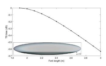
**Fig. 6.** TS bias (underestimation) plotted as a function of BFT fork length for a pulse duration of 64  $\mu$ s. The inset shows the geometrical scheme of the insonified volume for a pulse duration of value  $\tau$ .
