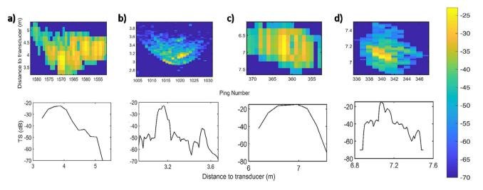
**Fig. 8.** a) Echogram trace of a single tuna (above) and temporal envelope of the ping with maximum echo TS within (below); 1024 µs pulse duration and acoustic beam size of 31° (Simrad ES10 at 200 kHz). b) Trace and envelope for 64 µs pulse duration for the same beam size of 31° c) Trace and envelope for 1024 µs pulse duration and acoustic beam size of 7° (Simrad ES200-7C at 200 kHz), d) Trace and envelope for 64 µs pulse duration for the same beam size of 7°.
