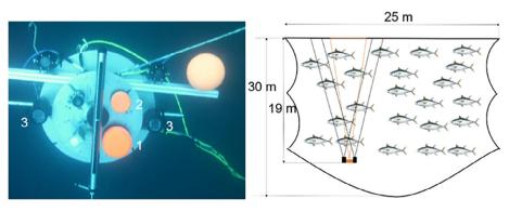
Fig. 1. Experimental setup. Underwater platform (left) 120 kHz transducer (1), 200 kHz transducer (2) and stereoscopic camera system (3). Setup diagram (right): Equipment at the bottom facing the surface.
