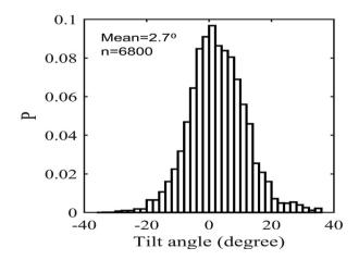
Fig. 10. Swimming tilt angle of the ABFT obtained from optical system for all acoustic-optical correspondences found at 120 and 200 kHz.
