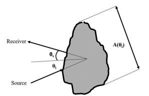
Fig. 5. Scheme of incident and scattering directions  $(\theta_{i,}\ \theta_{s})$  and apparent cross-section A( $\theta_{i}).$
