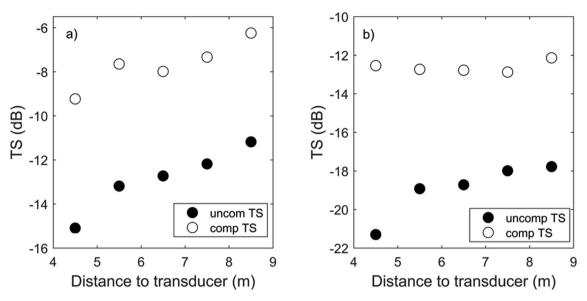
Fig. 12. Plot of TS versus depth for the 220 to 230 cm group of tuna length: a) 120 kHz data; b) 200 kHz data.
