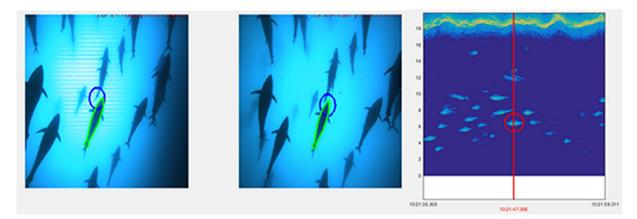
Fig. 4. Data processing image: On the left, images from stereoscopic system, the blue circle corresponds with acoustic beam. Straight tuna crossing the acoustic beam is measured. On the right we can see an echogram, the red line marks the acoustic trace corresponding with images (red circle). (For interpretation of the references to colour in this figure legend, the reader is referred to the web version of this article.)
