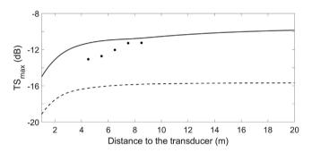
**Fig. 13.** Maximum TS calculated from the swimbladder model at f = 120 kHz for FL = 120 cm (solid) and FL = 200 cm and uncompensated TS measured for fork length between 220 and 230 cm at 120 kHz (dots).
