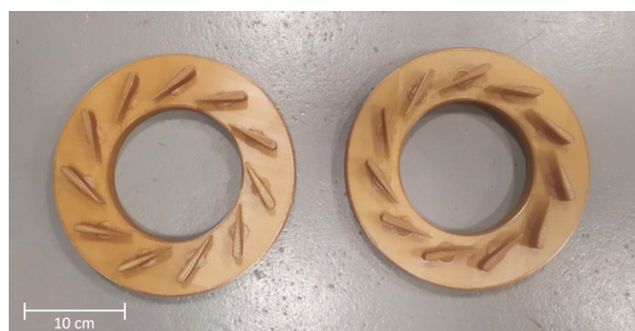
Figure 1. Printed nozzles with different vanes position.
