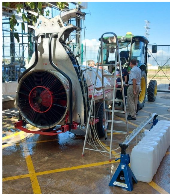
Figure 1. Laboratory evaluation of a modified blast sprayer.
