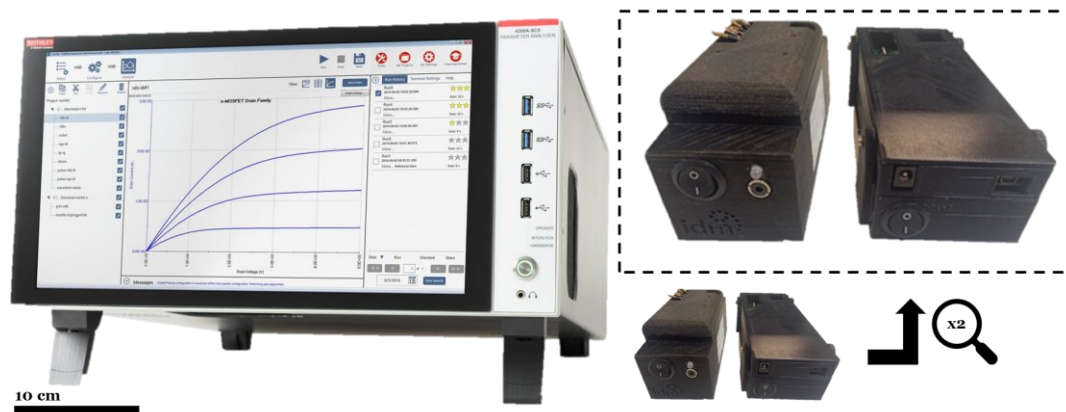
Figure 242. Left: Keithley 4200A-SCS from Tektronix official webpage 27 . Right: MBMS (right) and its predecessor (left) to scale, with the Parameter Analyzer, and with x2 amplification.
