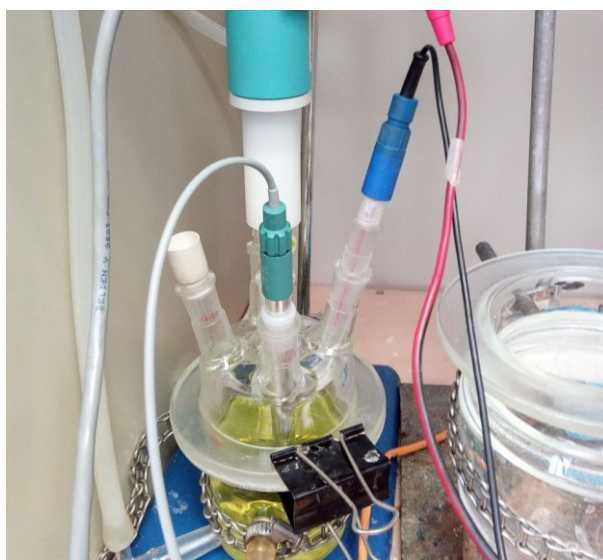
Figure 86. Electrochemical cell and solution for electrochemical validation of FAEVIS compared to Metrohm Autolab.
