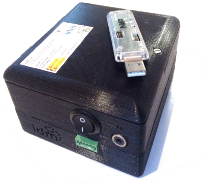
Figure 66. FAEVIS appearance, in PLA 3-D printed by parts box, with JACK battery charger socket, turn on button and signal PHOENIX connector.
