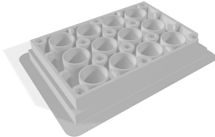
Figure 142. 3D-printed PLA 24-well matrix with M4 holes for screwing it to a PMMA lamina.
