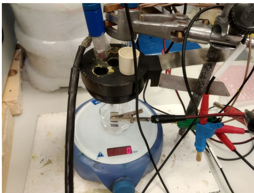
Figure 106. Electrochemical cell setup for the characterization of C2 reduction under P3 conditions.
