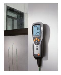
Figure 7. Thermal transmittance measure device, model Testo 435
