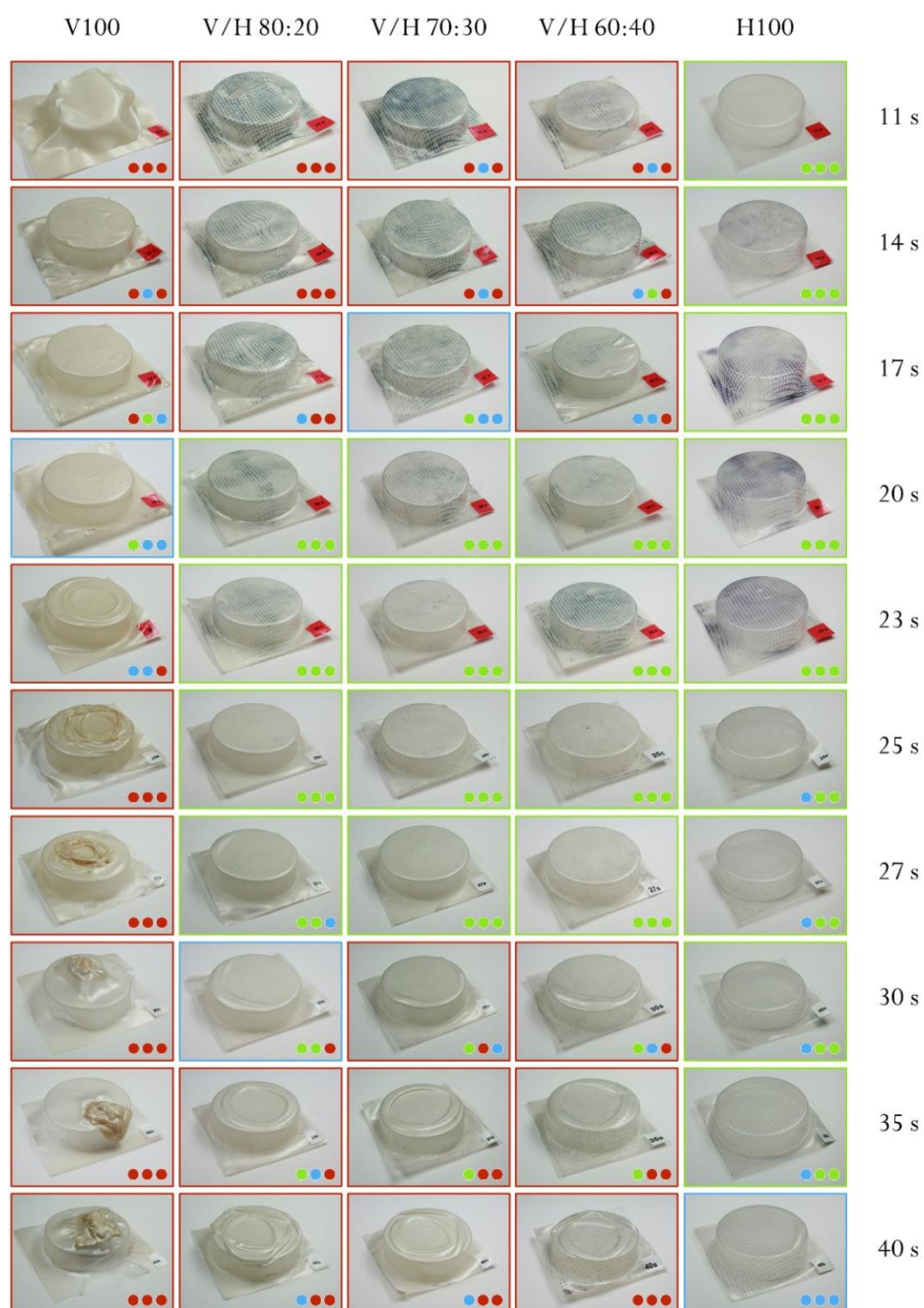
Figure 11. Photographs and evaluation of the thermoformed structures of poly(3-hydroxybutyrate-co-3-valerate) (PHBV), poly(3-hydroxybutyrate-co-3-hydroxyhexanoate) (PHBH), and their blends
