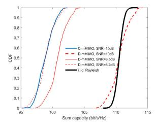
**FIGURE 11.** Analysis of the reduction of the SNR achieved with the D-mMIMO system, considering active the 20 UTs.
