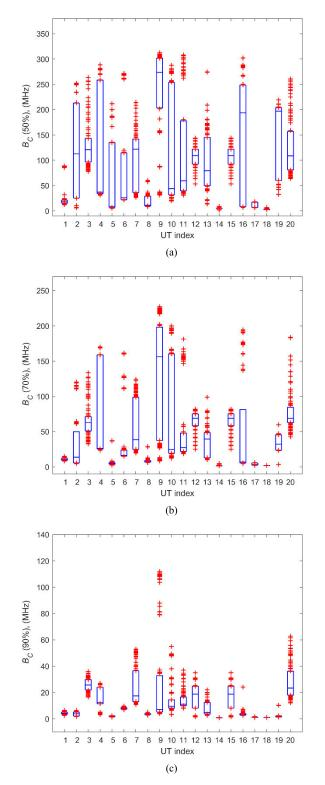
FIGURE 5. C-mMIMO individual coherence bandwidth values experienced by the 20 UTs and different correlation levels: (a) 50%, (b) 70% and (c) 90%.
