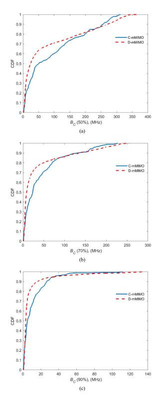
**FIGURE 4.** CDF of the coherence bandwidth values obtained when considering the whole set of 20 active Tx and comparing both mMIMO systems for different correlation levels. (a) 50%. (b) 70%. (c) 90%.
