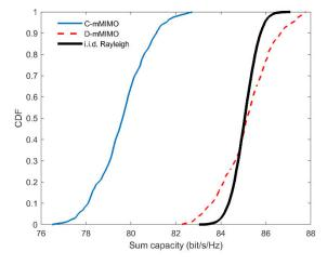
FIGURE 8. CDF of the sum capacity for C-mMIMO and D-mMIMO systems and 15 active users or Tx (Tx: 1-2, 4-5, 7-11, 13-16, 18-19).
