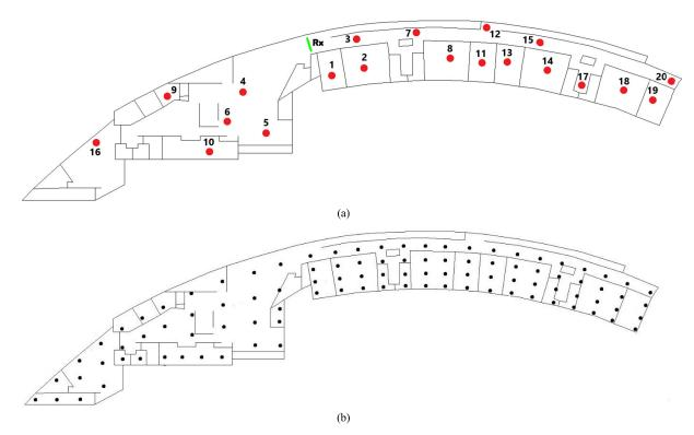
FIGURE 3. Transmitters and receivers locations for C-mMIMO and D-mMIMO. (a) Distribution of the 20 Tx/users on the site. Details of both location and orientation of the receiver array for the C-mMIMO case are included. (b) Distribution of the 100 Rx antennas for the D-mMIMO situation.
