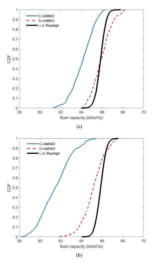
**FIGURE 7.** CDF of the sum capacity for C-mMIMO and D-mMIMO systems and 10 active users or Tx in two situations. (a) Dispersed Tx (Tx: 1, 3-4, 8, 10, 12, 15-17, 20). (b) Nearby Tx (Tx: 8, 11-15, 17-20).
