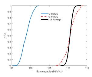
**FIGURE 9.** CDF of the sum capacity for C-mMIMO and D-mMIMO systems and considering active all the 20 users or Tx.
