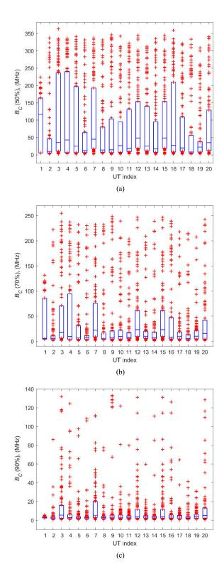
FIGURE 6. D-mMIMO individual coherence bandwidth values experienced by the 20 UTs and different correlation levels: (a) 50%, (b) 70% and (c) 90%.
