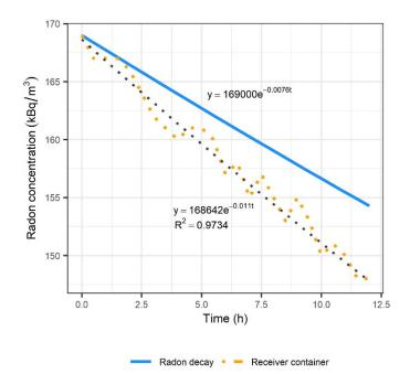
Figure 5. Radon leakage test performed in the receiver container
