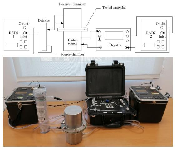
Figure 1. Experimental system set-up.
