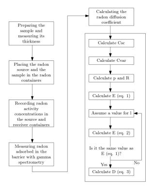
Figure 3. Flow chart of the measurement process and calculation of the radon diffusion coefficient
