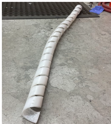
Figure [18] HDPE extracted from the Screw after Purging Process
