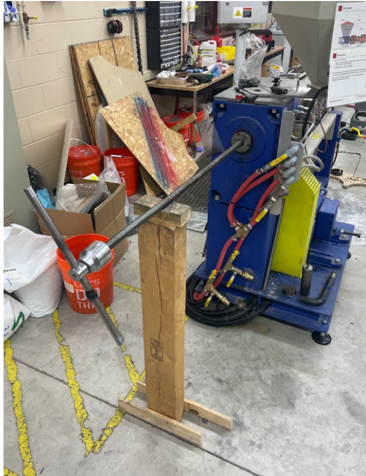
Figure [14] M24 precision screw extractor supported by wooden stand
