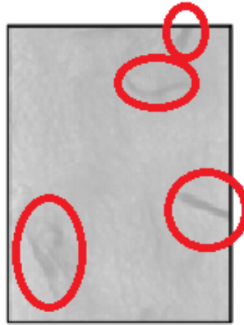
Figure [24] Observable Fiber Dispersion
