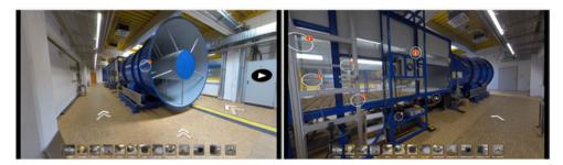
Figure 1. 3D virtual representation of the Boundary Layer Wind Tunnel at the Ruhr-Universität Bochum - remote access points are marked "i" and show explanations about steering and sensoring of experiments as well as videos of specific experiments; experimental parameters can be varied within a certain range, corresponding data from previous experimental campaigns can be downloaded for further processing.
