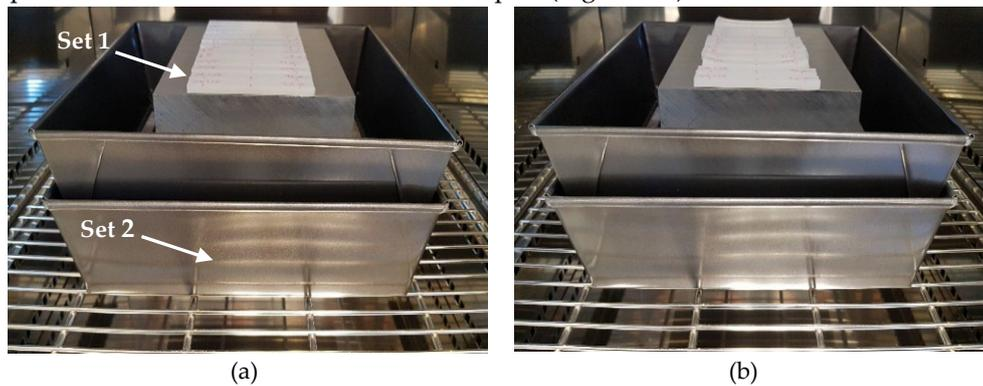
**Figure 4.5.** (a) Samples before thermal treatment in the furnace; (b) after thermal process, deformation is clearly visible in samples of Set 1.
