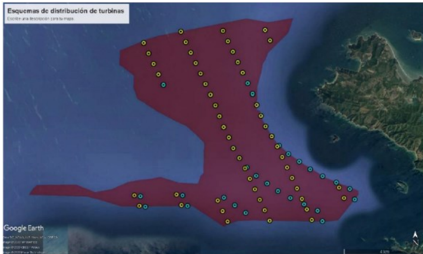
Figure 3.2 Wind turbine layout options (A in yellow, B in cyan). Adapted from [33]
