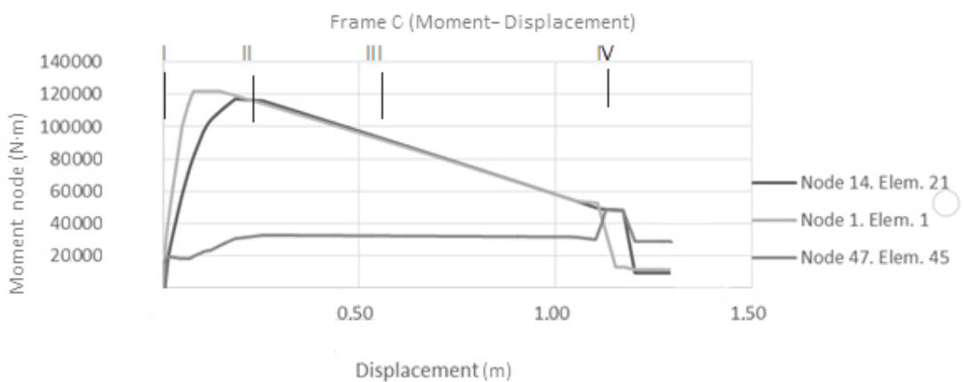
Figure 24. Graph of the moments in elements 1 and 24 front the displacement in Node 14 of frame C.
