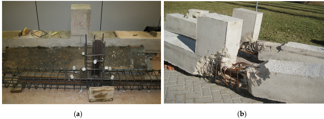
Figure 1. Prototypes P03 and P04 in the execution phase (a) and image of the tested prototypes P03 and P04 (b) [17].
