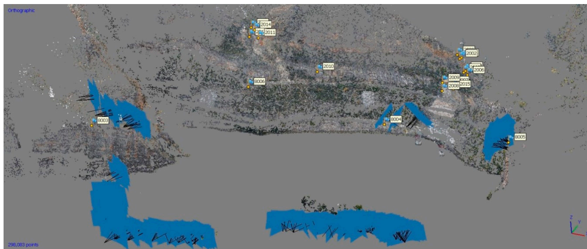
Figure 5. Set of imagery used for the bundle adjustment of the normal and tele cameras and visualization of the measured points on geodetic pillars and check points.
