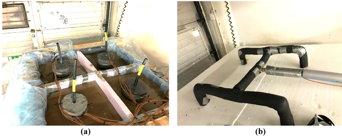
Fig. 7. The four-column test setup: (a) Four separated columns filled with sand and saturated with water, and (b) Connection of the grout columns to the circulation pump.
