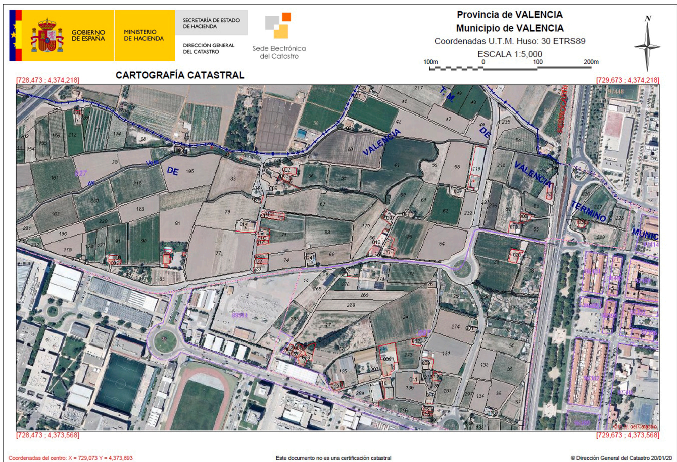
Fig. 1. Example of a cadastre electronic office map for printing based on orthophotography from the National Aerial Orthophotography Plan (PNOA), 2020. Source: DGC
