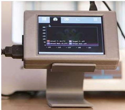
Figura 71: Panel de control impresora 3D. [99]
