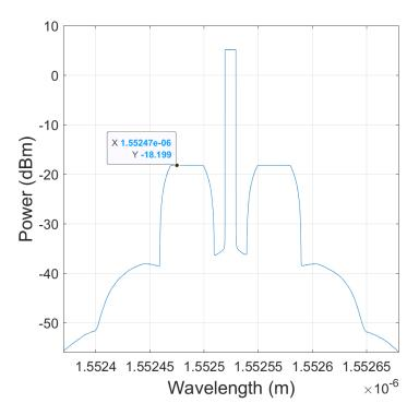
Figure 3.11: Optical Spectrum emitted by a fixed laser
