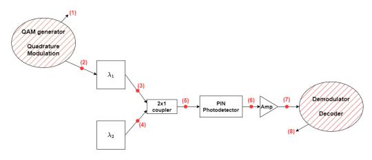
Figure 3.9: System overview using Optisystem
