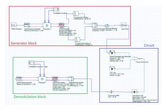
Figure 3.4: System overview using Optisystem
