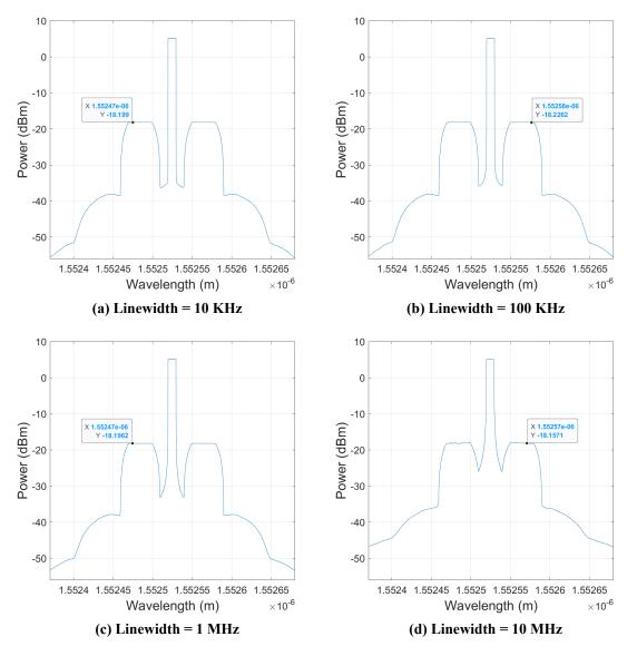
Figure 3.17: Optical spectrum after the fixed laser for 5.299 dBm output power, 100 GHz frequency and different linewidth values
