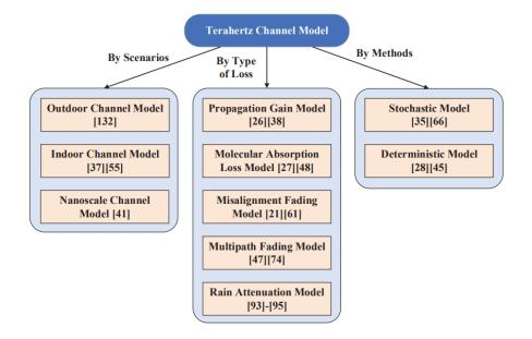
Figure 2.3: Channel model classification for THz band [16]
