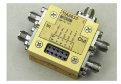
Figure 2.17: Limiting amplifier by Micram
