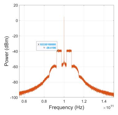
Figure 3.15: RF Spectrum after Amplifier
