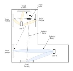
Figure 2.20: Smart surfaces system [36]
