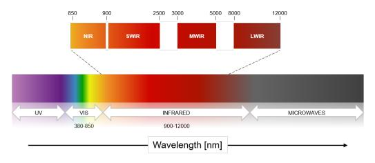
Figure 2.2: Infrared band [14]
