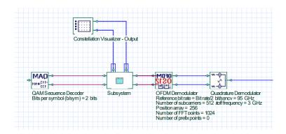
Figure 3.7: Overview of the output constellation visualizer
