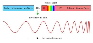
Figure 2.1: Radio spectrum [12]
