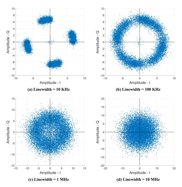
Figure 3.16: Output constellation for 5.299 dBm output power, 100 GHz frequency and different linewidth values
