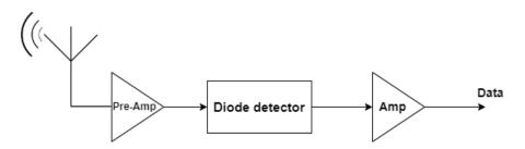
Figure 2.15: Receiver block diagram
