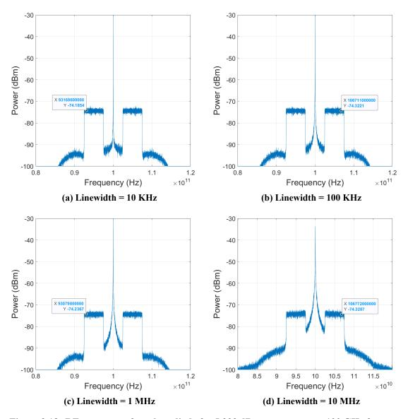
Figure 3.18: RF spectrum after photodiode for 5.299 dBm output power, 100 GHz frequency and different linewidth values
