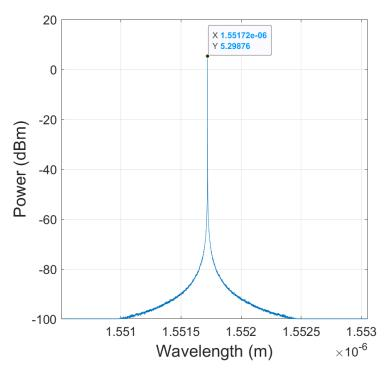
Figure 3.12: Optical Spectrum emitted by variable laser
