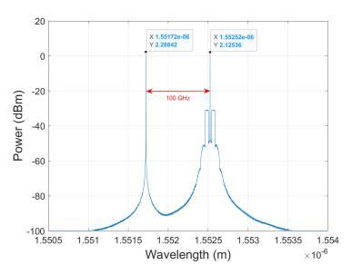
Figure 3.13: Optical Spectrum after combination of both Lasers
