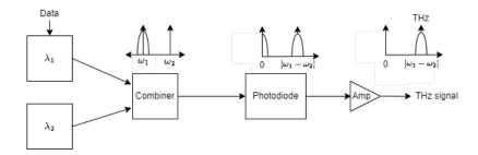
Figure 2.6: Simple scheme for photonic generation of THz signals using two lasers
