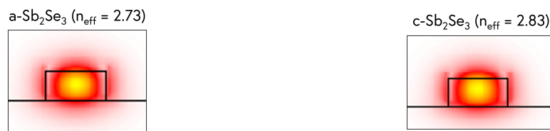
Figure 2.15: Mode of the waveguide with a width of 450 nm at amorphous state.
