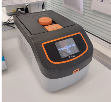
Figure 4.6: TECHNÉ 3Prime Thermal Cycler (thermocycler).
