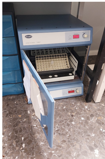
Figure 4.9: Stuart SI500 orbital shaker incubator.
