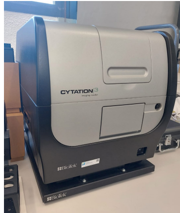
Figure 4.8: Cytation 3 Imaging Reader by Agilent Technologies.
