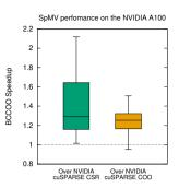
Figure 6. Speedup analysis comparing the performance of the BCCOO SPMV against the COO SPMV and the CSR SPMV from NVIDIA's cuSPARSE library on the NVIDIA V100 (left) and NVIDIA A100 (right).
