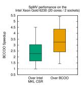
Figure 8. Speedup analysis comparing the performance of the BCCOO SPMV against Intel's CSR SPMV and the BCOO SPMV on the Intel Xeon Gold 6230.
