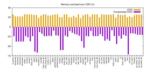
Figure 3. Memory overhead of the multicore CPU version of the compressed COO format taking the CSR format as baseline. All data is assumed to be stored in DP.
