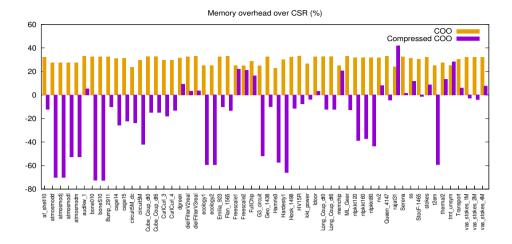
Figure 1. Memory overhead of the many-core GPU version of the compressed COO formats taking the CSR format as baseline. All data is assumed to be stored in DP.
